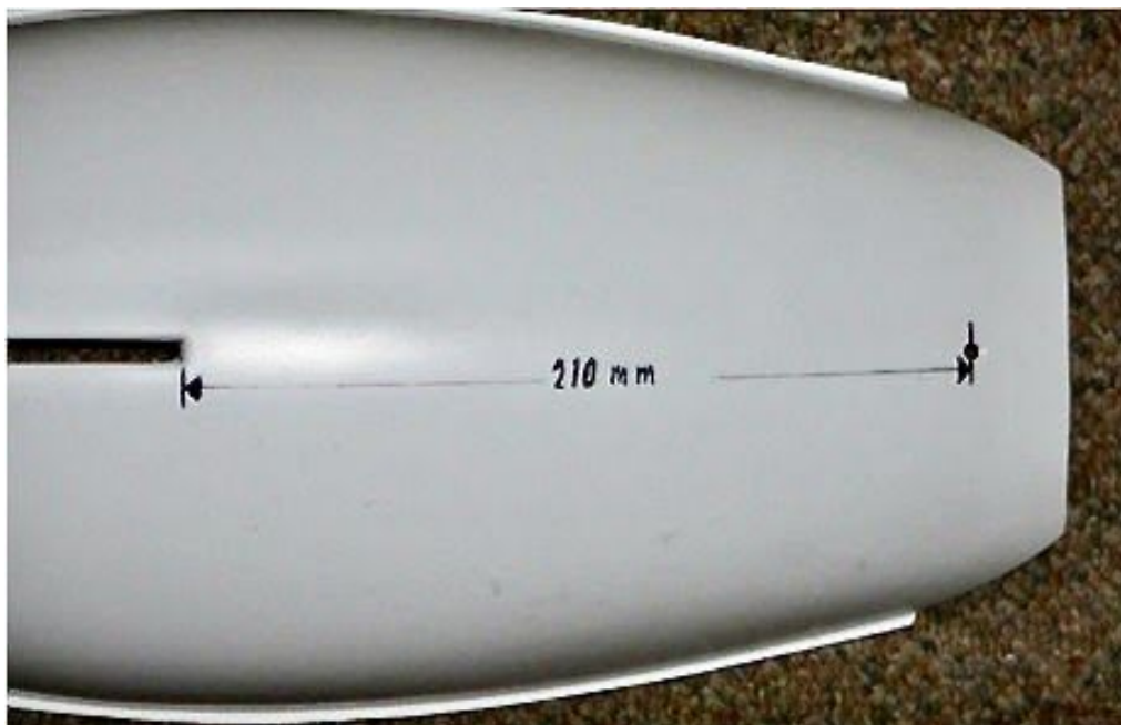
Figure 1: Position of Rudderpost on 2014.v2 Hulls
