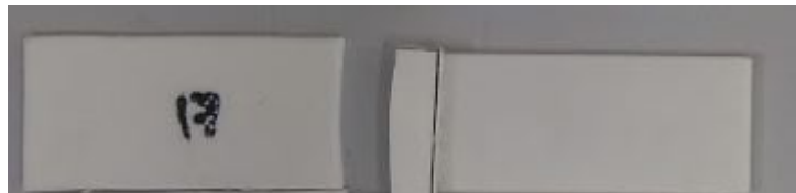
Sample where the material failed before the bond
